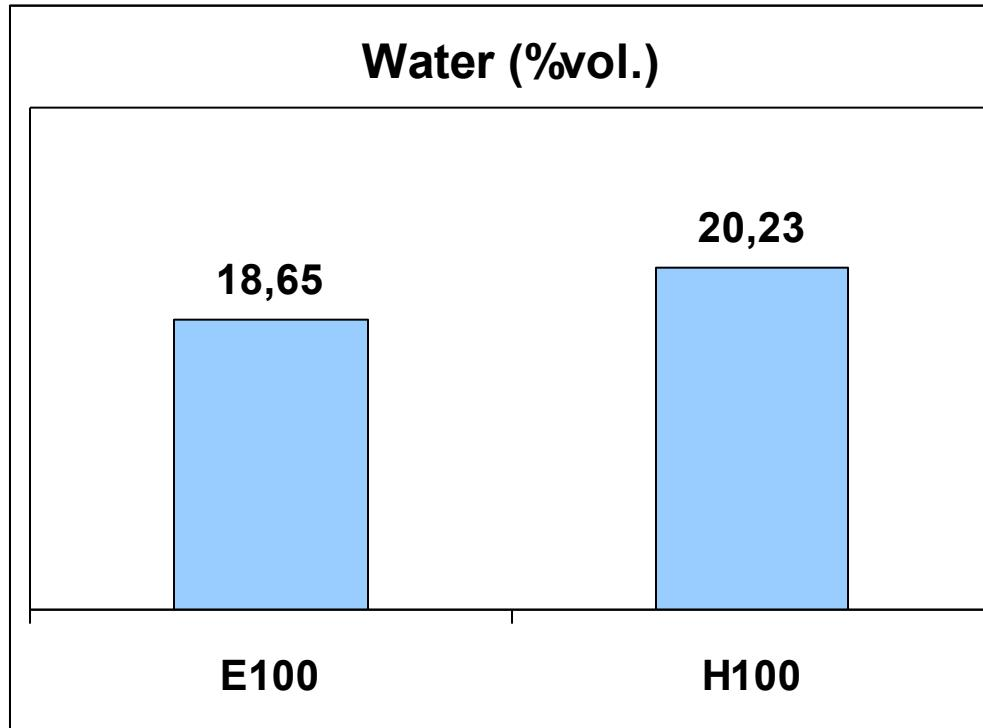
**E100 lower water proportion (%v.) in exhaust gases**
