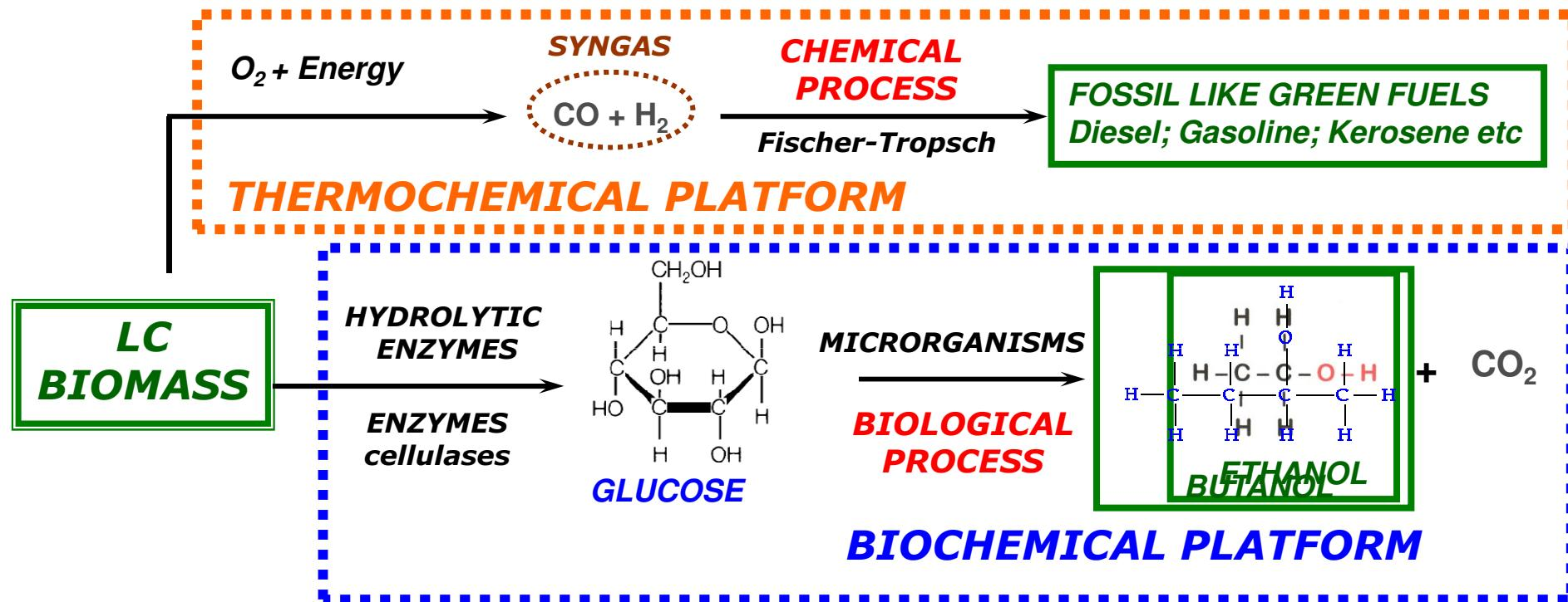
**Fischer-Tropsch** (1920) is a catalyzed chemical reaction in which carbon monoxide and hydrogen (syngas) are converted into liquid hydrocarbons of various forms (**Diesel, Gasoline, Kerosene e Lubricants**).
