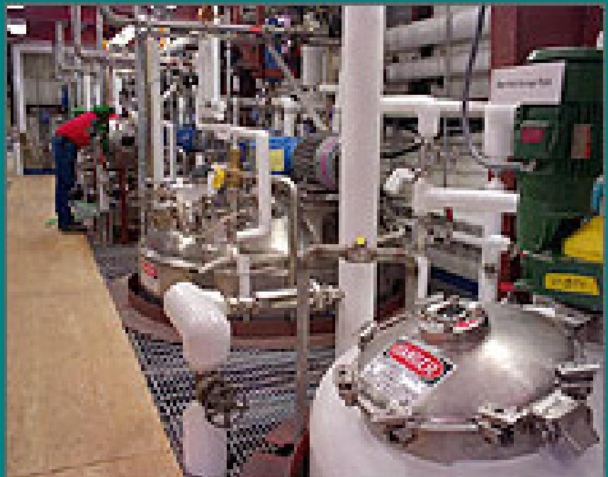
**04 bioreactors of 9.000 L; 02 of 1.450 L and 02 of 160 L (ethanol concentration = 30-40 g/L)**
