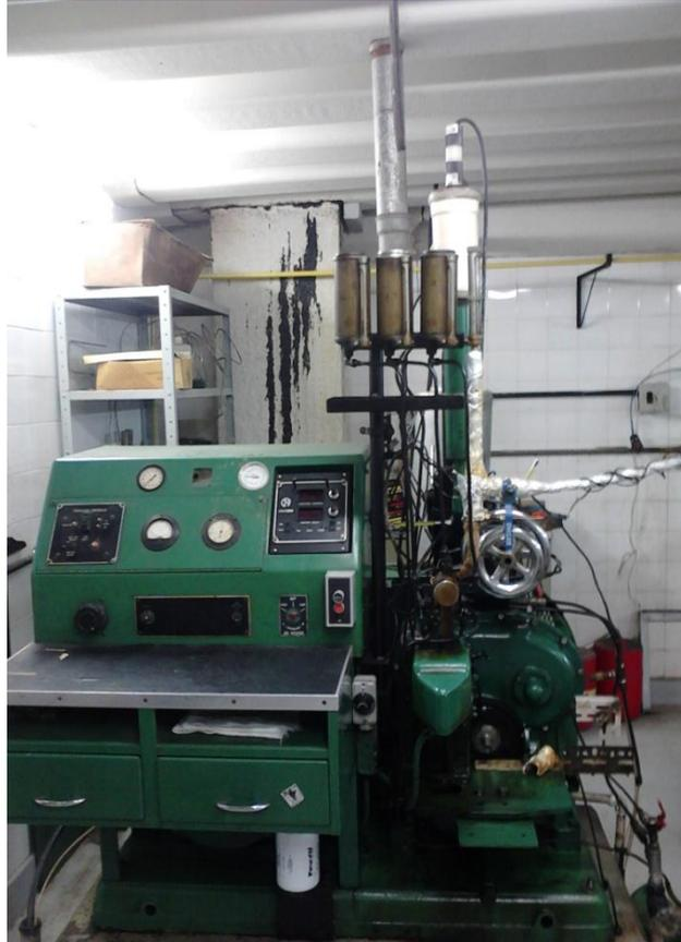
Figura 6.1 - Motor ASTM CFR Cetano
