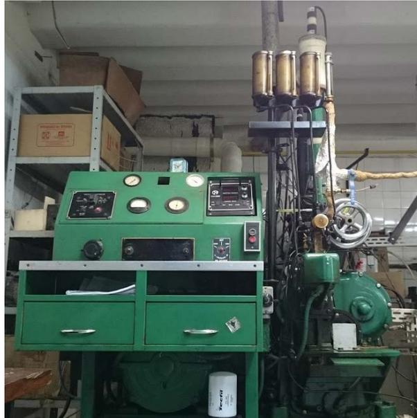
**Figura 10:** Motor ASTM CFR CETANO
