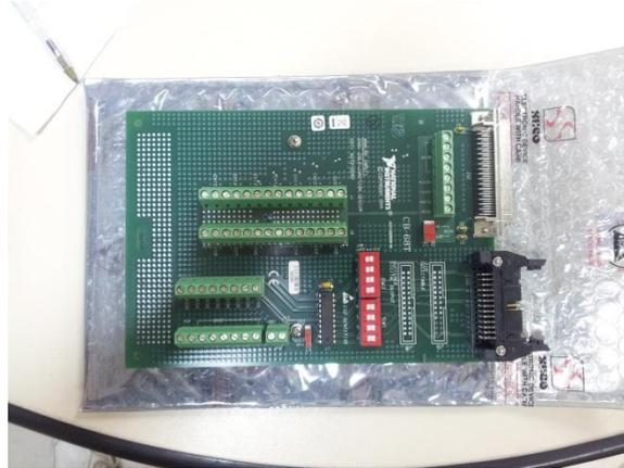
Figura 4.8. Bloco Terminal National Instruments CB-68T
